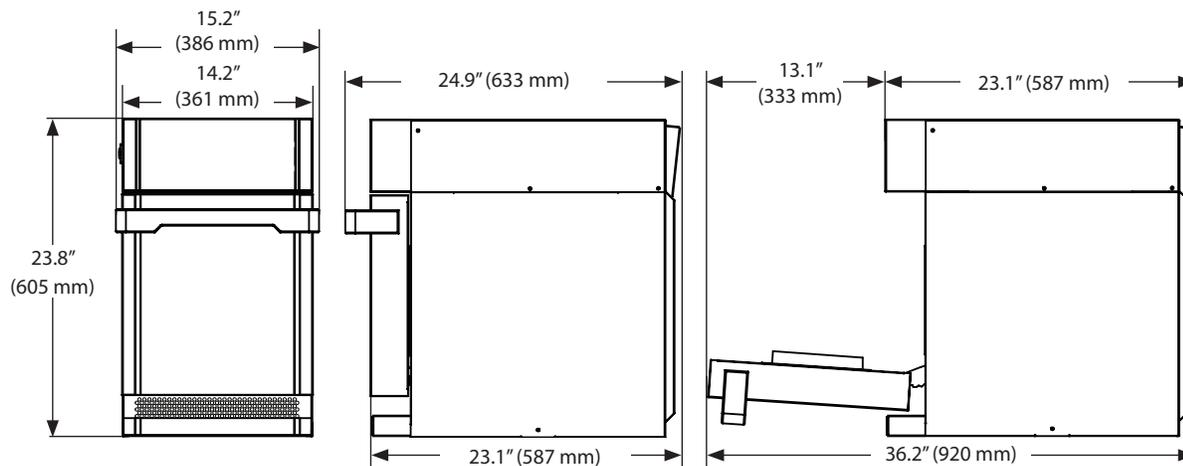
Figure 1: ECO ST Oven Dimensions
