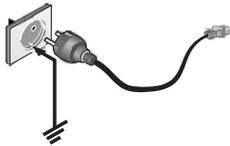
At the first start-up and after any period of inactivity longer than 8 hours without power (with the socket unplugged - button "8" off), you must **wait 1 hour and 30 minutes** with the refrigerating cabinet powered (socket plugged), before starting the compressor.
