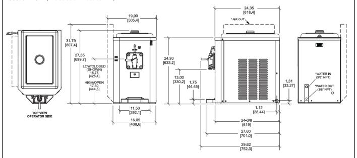
FIGURES IN BRACKETS INDICATE MILLIMETERS / DECIMAL DIMENSIONS EQUAL TO ( PLUS OR MINUS 1/16 INCH [1.5mm] ). \* WATER COOLED ONLY Shown with optional top air discharge chute.
